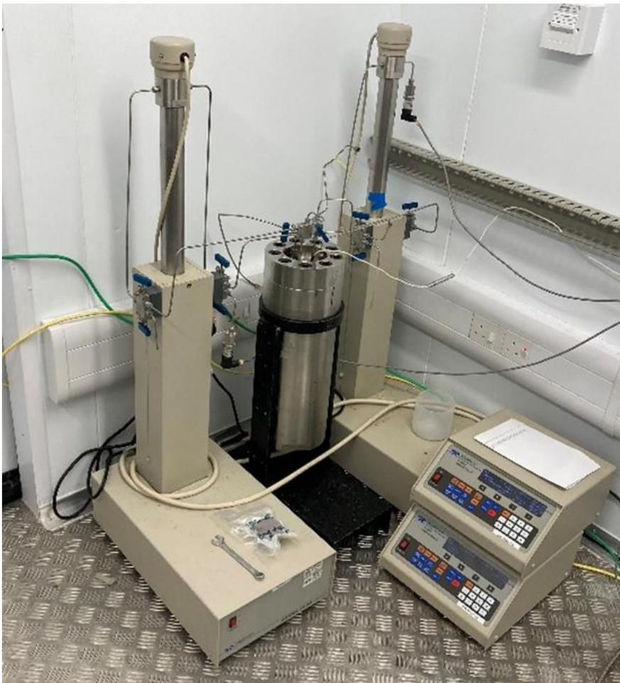
Figure 4-1 The pore pressure oscillation apparatus
